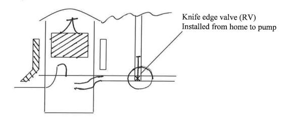
It is also recommended that heat tape circuit be installed around the candy cane, to reduce freeze up of the goose neck section. This can be done on all new installations. Older installations should review to add rigid Styrofoam inside the chamber OR place pink insulation above or just below lid (in a commercial garbage bag)
